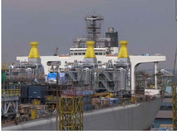
The boilers were lifted onto the FPSO Polvo by floating crane and fitted to the prepared bases on the vessel
